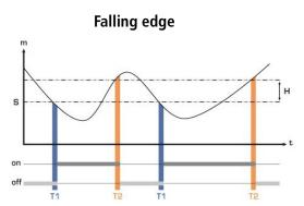
Measurement (m) < Threshold (S) during time-delay T1  $\rightarrow$  Alarm activation.
