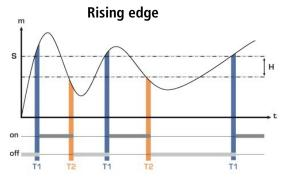
Measurement (m) > Threshold (S) during the timedelay T1  $\rightarrow$  Alarm activation Measurement (m) < Threshold (S) - Hysteresis (H) during the time-delay T2  $\rightarrow$  Alarm deactivation
