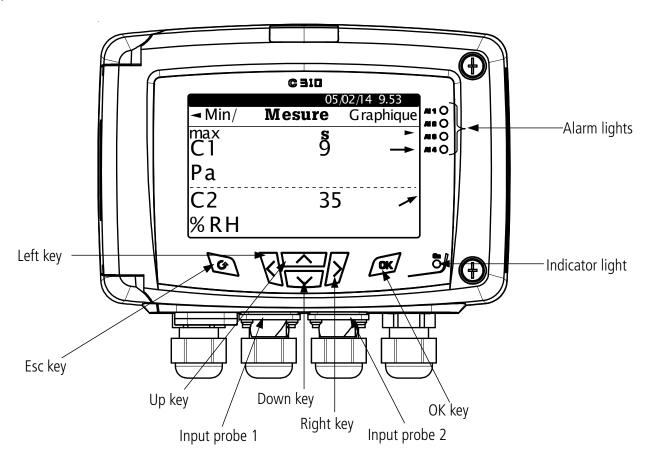
**Trend indicator:** on the screen, a trend indicator represented by a rising arrow, a going down arrow or a stable arrow is displayed above the measurement unit. It means the calculation of a moving average on the last hour (M1) to compare with a moving average on the last 5 minutes (M2):
