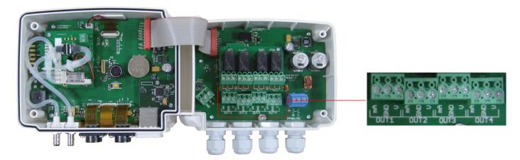
Connect a measurement device on the output 1, 2, 3\* or 4\*.
